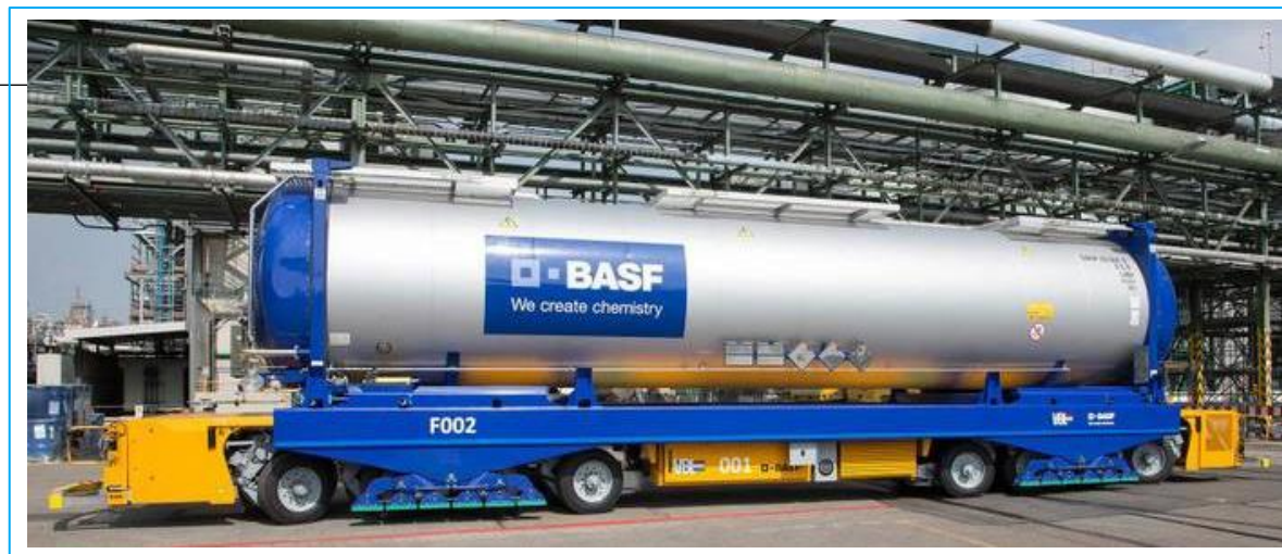
BASF & VDL's autonomous guided vehicle transports chemicals
